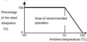
Figure-1 Derating curve
