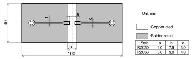
Figure-4 RZC50, 63 BOUND STRENGTH OF THE END FACE PLATING TEST SUBSTRATE
