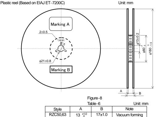
Note: Marking label shall be marked on a place of Marking A or two place of marking A and B.
