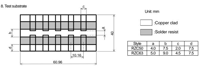
Figure-3 RZC50, 63 TEST SUBSTRATE
